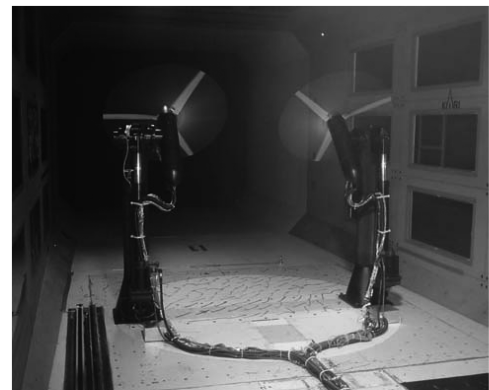
Fig. 6 Proprotor test rig installed in the wind tunnel.
